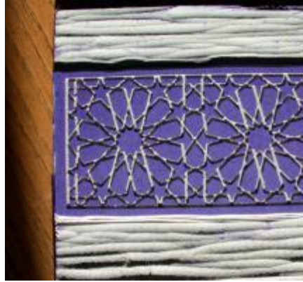
A linoleum block with a pattern cut by a 3-axis machine (the outside was carved away)
